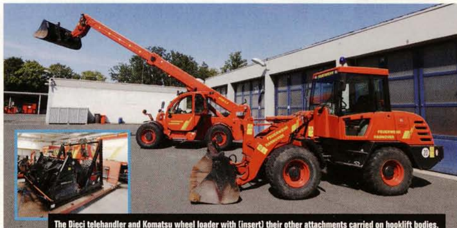
The Dieci telehandler and Komatsu wheel loader with (insert) their other attachments carried on hooklift bodies.
